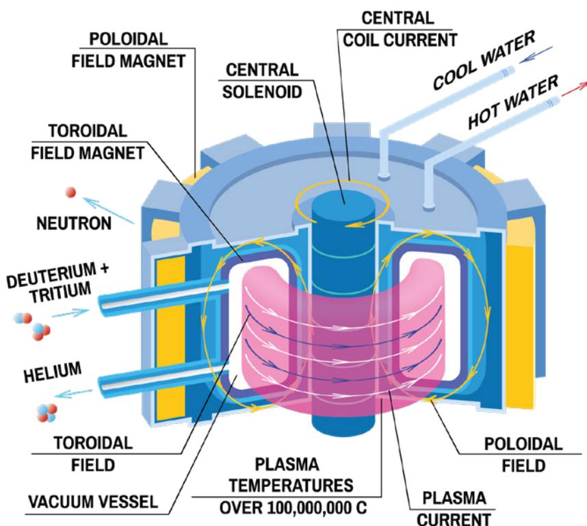
The **neutrons** that are generated can be captured by atoms in the reactor making them unstable and therefore **radioactive**. The reactor must therefore be **shielded** using concrete to prevent any radiation escaping and so protect the workers.
