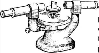
If you want to analyse light from stars or galaxies, you will need a **spectrometer**. This has a diffraction grating that splits all the different wavelengths up in a very precise way.
